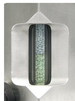
Figure 1. Polycarbonate shield surrounds the glass indicator.
